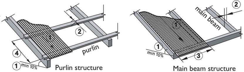
Calculation of maximum recommended\* distance between main beams and between purlins for **flat roofing** must take into account wind pressure of up to 100 kg/m<sup>2</sup>.
