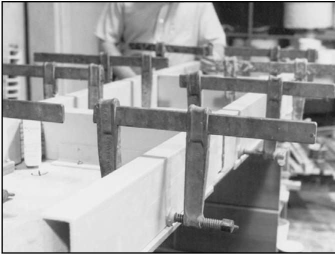
6. Appropriately clamp assembly to hold secure while the adhesive cures.
