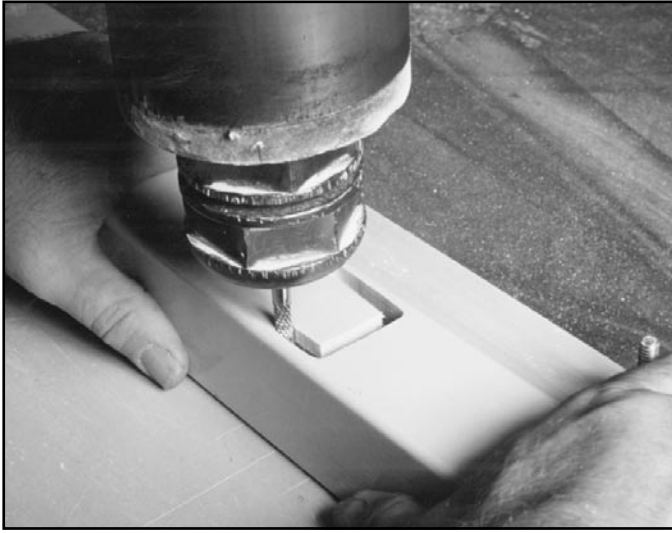
A stationary router is particularly useful for cutting keyways, slots and for performing other milling operations.
