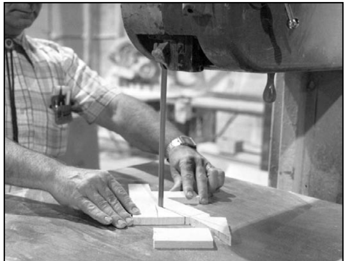
A band saw is ideal for cutting circles, irregular shapes and large shapes.
