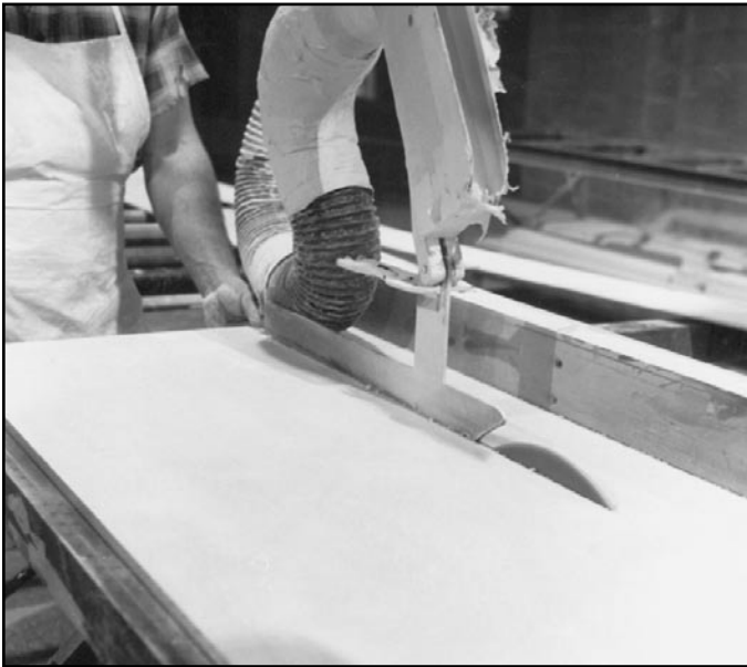
Straight line sawing (vacuum hood raised).
