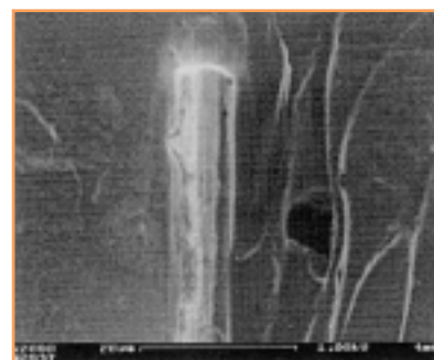
Conventional carbon fiber filler (on right) shows rough surface and individual fiber pull out.
