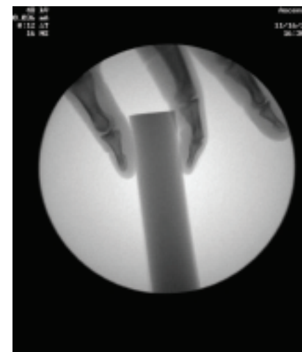
TECAPEEK™ Classix™ XRO™ Radio Opaque materials are clearly visible on X-rays.
