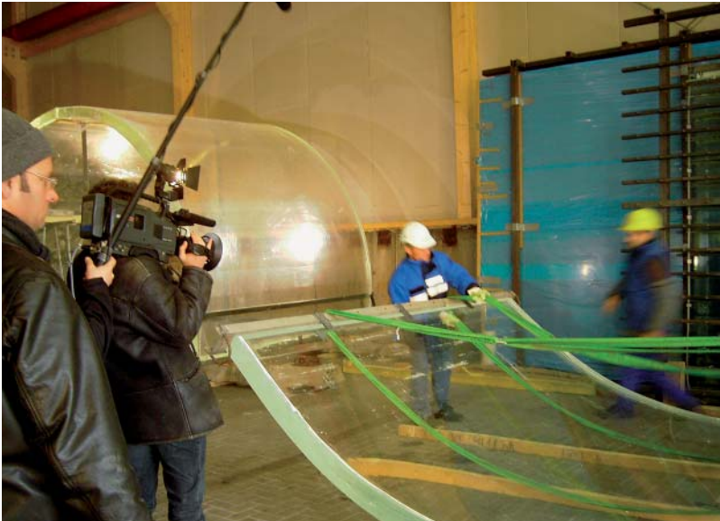
Biacryl in Halle forms and bonds the giant ACRYLITE® blocks into uniform tunnel vault segments. Then off they go to Gelsenkirchen Zoo, to delight sea lions and entrance watching children.
